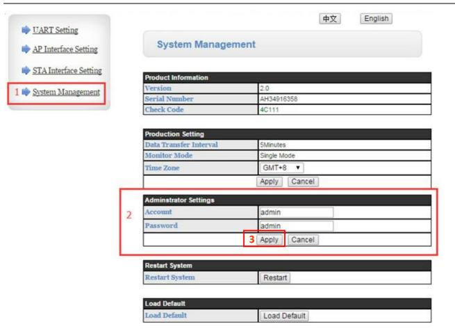
From year 2015, "AH" WiFi model with FW version 4.0, password of personal router is invisible from WiFi interface setting page, as below picture, this is another way to protect customer's information security. Older WiFi module can be update to FW Version 4.0.
